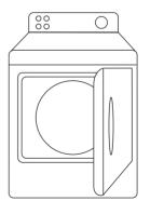
Power rating = 2400 Watts Running cost: 34p (per hour)
